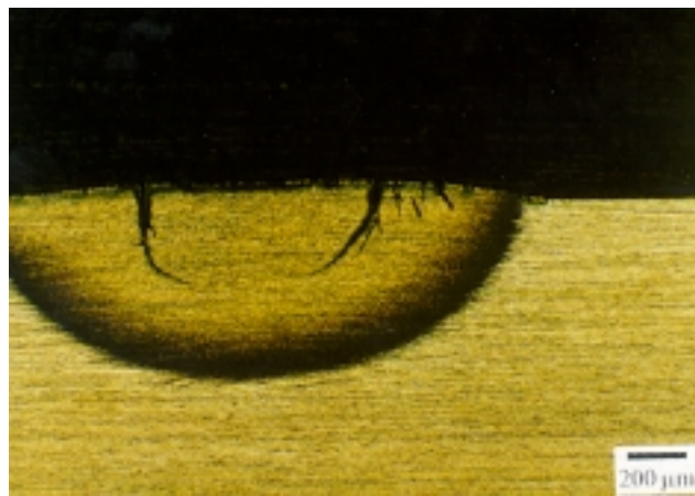
Fig. 7. Typical cross-sectional view of hydride blister.
