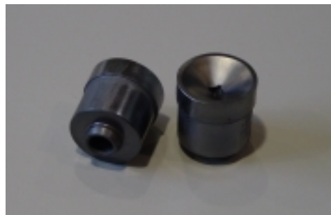
Fig. 2. Photograph of die for Indirect co-extrusion.
