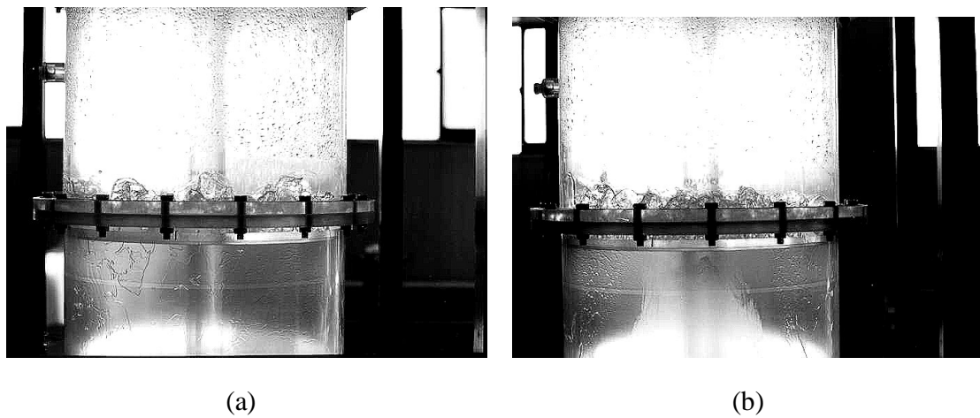
(a) (b) Figure 5. Fully limiting CCFL (1 mm gap, j_L^{*1/2}=1.152 )
