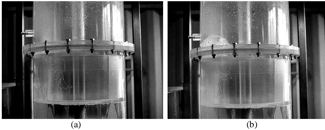
(a) (b) Figure 4. Partially limiting CCFL (1 mm gap, j_L^{*1/2}=1.152 )
