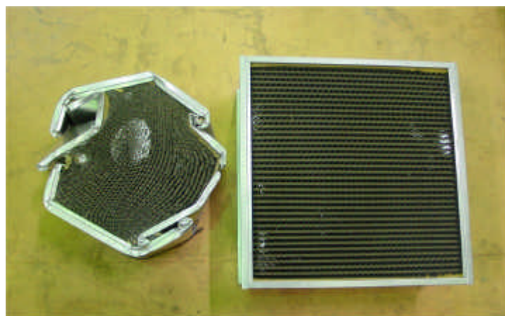
Fig. 6 Used HEPA Filter Waste Before(Right) and After Compaction(Left)
