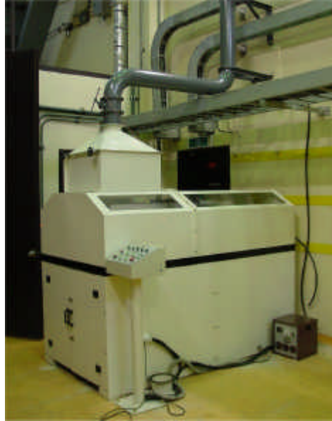
Fig. 5 Used HEPA Filter Compactor Developed by KAERI
