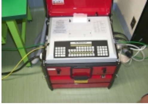
(a) Welding control console
