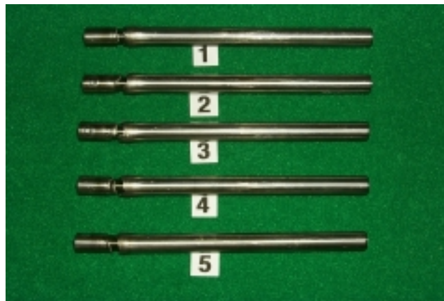
Fig. 3.3 End plug burst fractured specimens
