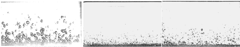
Boiling at low subcooling / Boiling at higher subcooling/ DNB at higher subcooling
