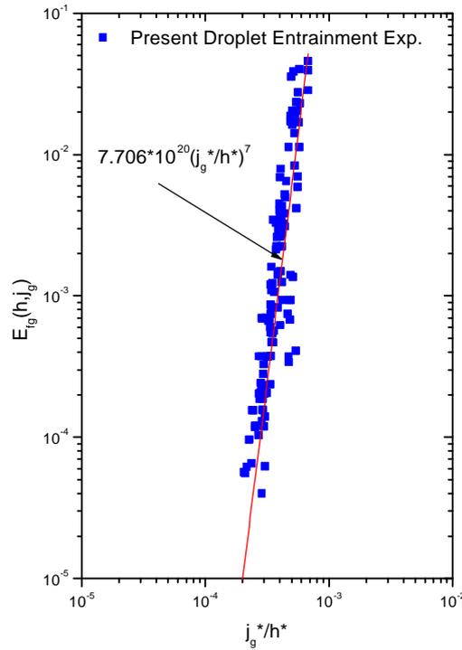
Fig. 3 Present entrainment data in plot of  $E_{fg}$  versus  $j_g^*/h^*$ .
