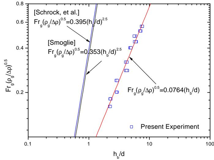
Fig.6 Comparison of the present off-take data with the existing correlations for the horizontal pipe with top break.
