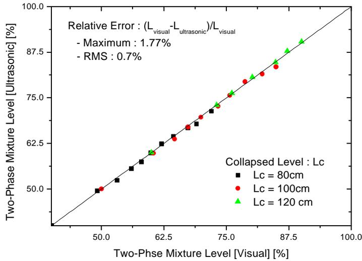
Fig. 2 Comparison of ultrasonic sensor data with visual level data.
