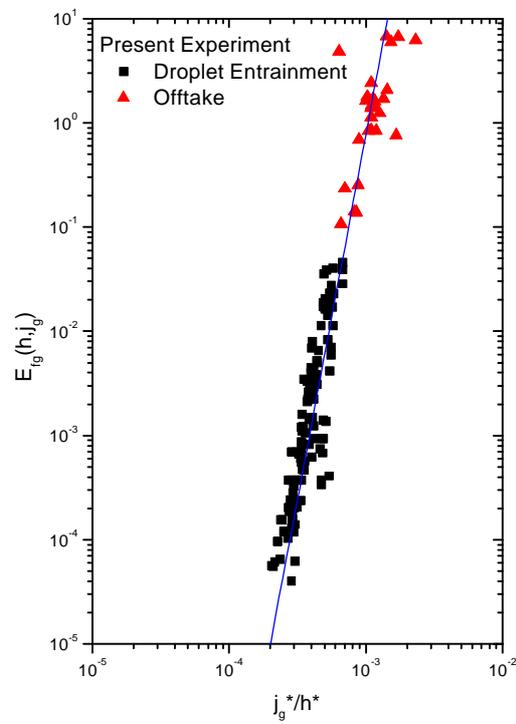
Fig. 8 Present entrainment and off-take data in plot of  $E_{fg}$  versus  $j_g^*/h^*$ .
