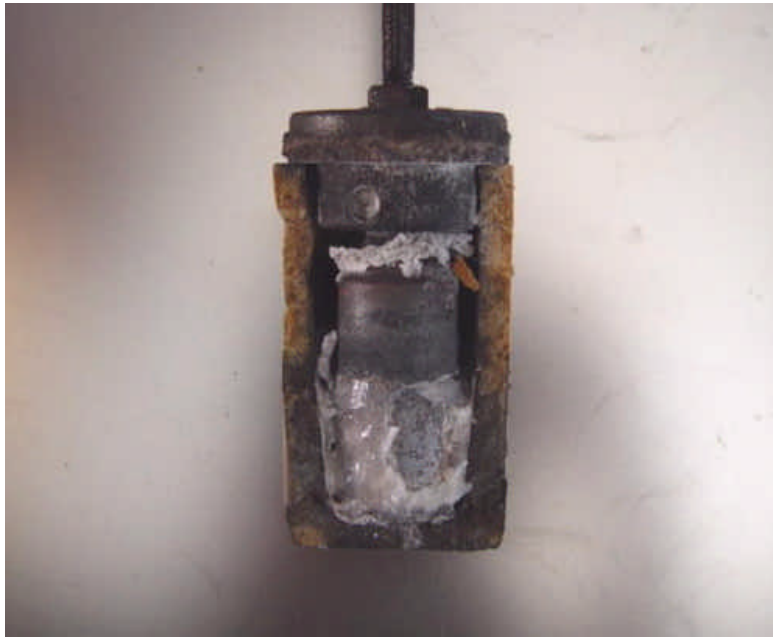
Fig. 2. Li in MgO container.
