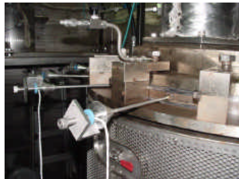
Fig.5 AE Sensors and Waveguides Mounted
