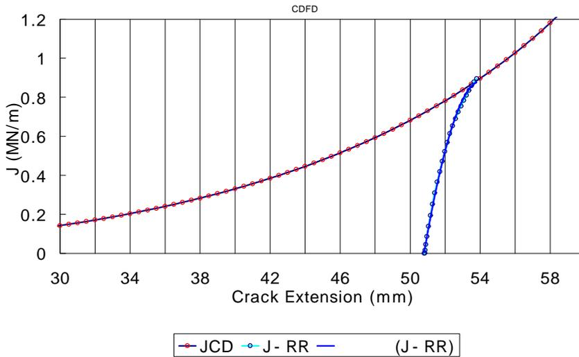
Fig. 6 Determination of CCL (Zr-03/25 ) using JCDF
