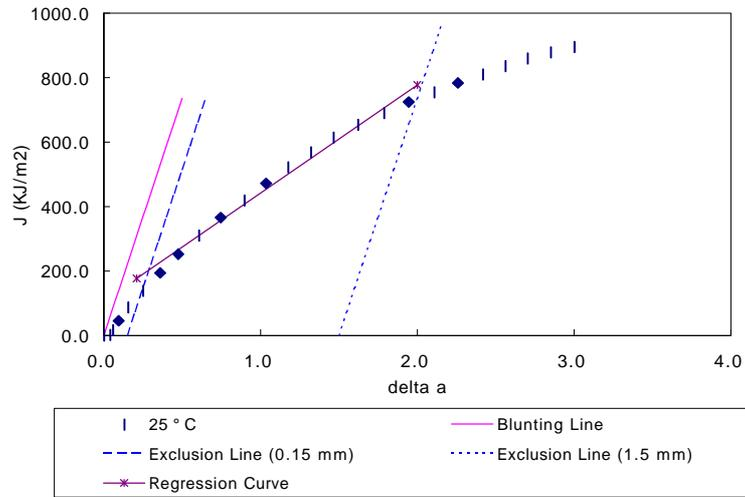
Fig.3 Typical crack resistance curve at room temperature
