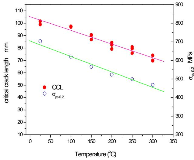
Fig. 7 CCL and yielding strength ( $\sigma_{ys,0.2}$ ) comparison with various temperature
