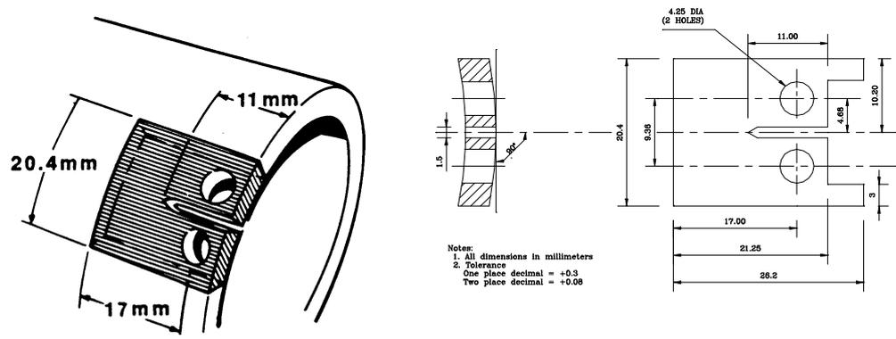
(b) Geometry of CCT Specimen
