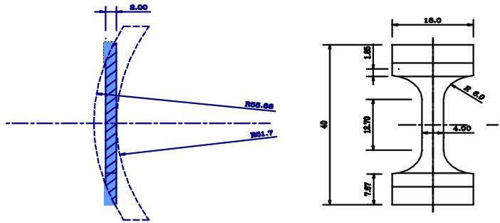
(a) Geometry of transverse tensile specimen
