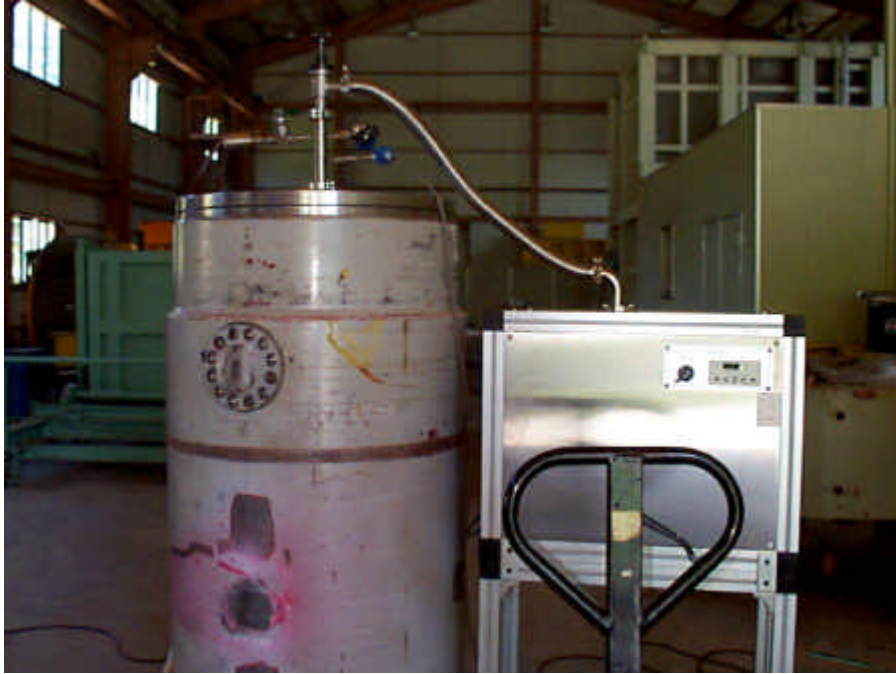
Fig. 5. Leak Test before Water Immersion.
