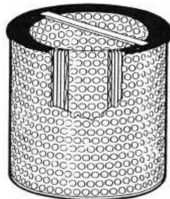
Fig. 6 cylindrical filter of hot-cell exhaust
