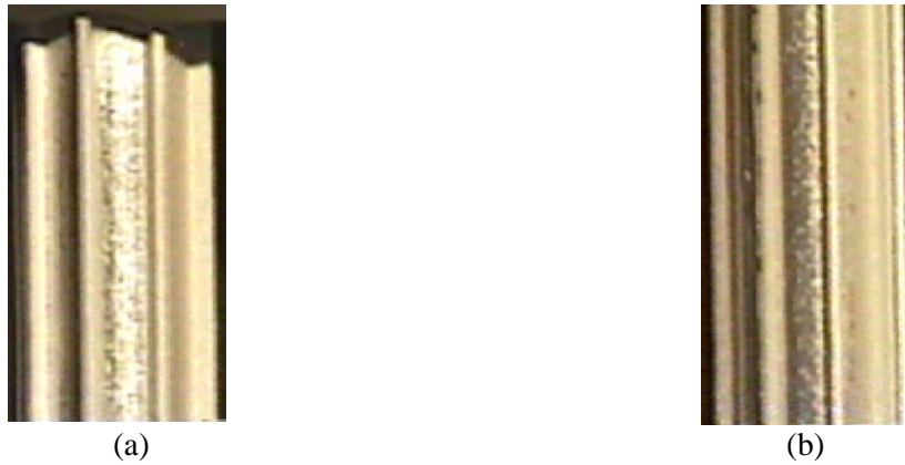
Fig. 6. Photograph showing the longish cleavage-like defect on cladding in the region fuel rod having the linear power of 80 KW/m(a) and 107 KW/m (b).
