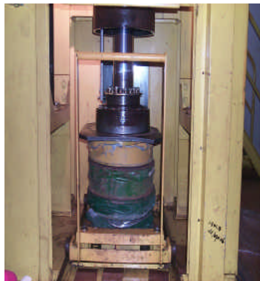
Fig. 5. Under Compacting of Spent Drum
