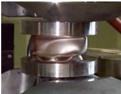
Fig. 9 Crush test of cylindrical thin-walled tube ( L/D=1.25 ).
