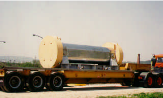
Fig. 1 Configuration of a spent fuel transport cask.
