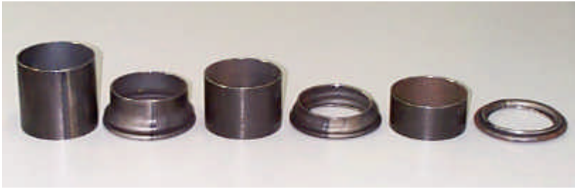
Fig. 7. Axisymmetric concertina buckling of cylindrical tubes. ( D = 90.0 , t = 2.0 )
