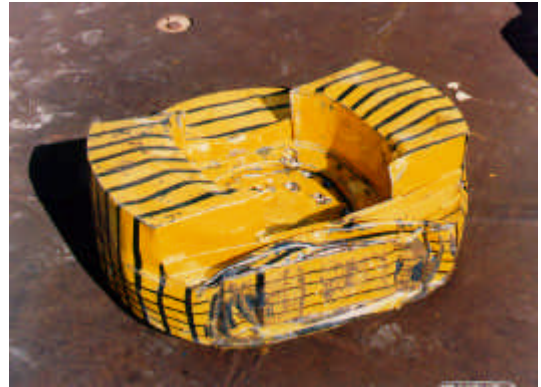
Fig. 2 Deformed shape of a cask impact limiter.
