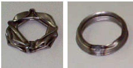
(a) fully butt-welded specimen
