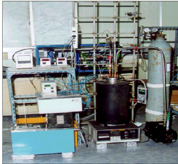
Fig.3 Photography of Experimental Apparatus for Vacuum Distillation.
