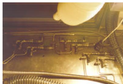
b) arrangement of pneumatic control valves
