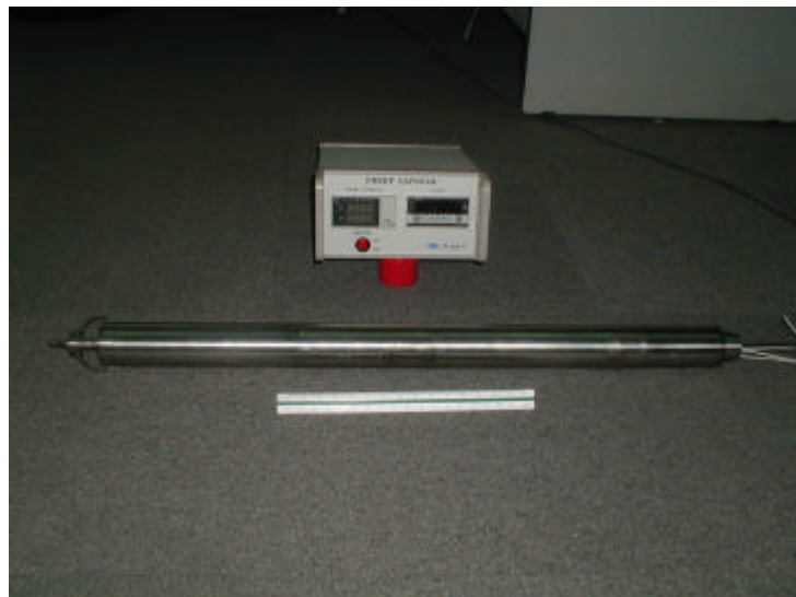
Fig. 2. Photo of in-pile creep capsule and controller
