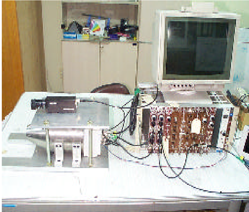
Figure. 2 The developed gamma camera system
