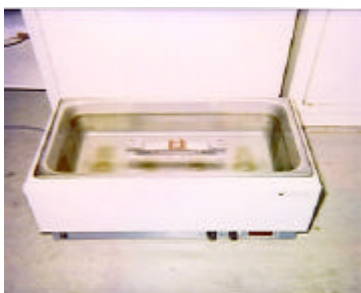
Fig. 3. SCC test in the thermostat at 40 °C
