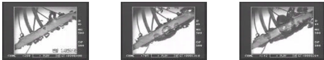
Fig. 2 Bubble Behavior at 30° Inclined Plate of W3L10 (98, 492 and 800 kW/m²)
