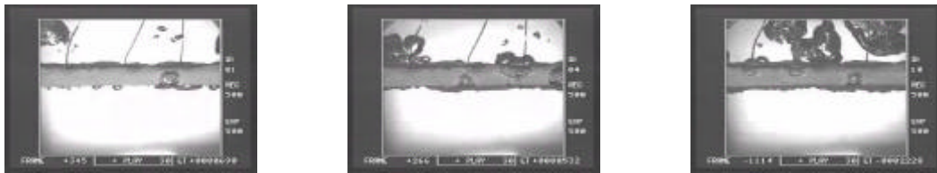
Fig. 1 Bubble Behavior at 0° Inclined Plate of W4L20 (50, 200 and 500 kW/m²)
