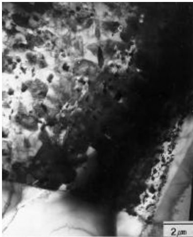
Fig. 7. Transmission electron microscopy analysis of the C14 alloy aged at 650°C
