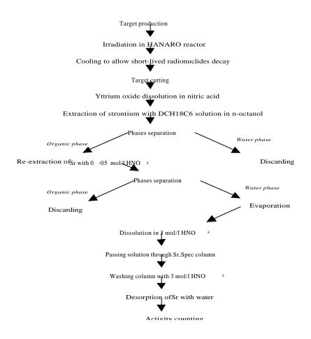
Fig. 1. The flow-sheet of extraction - based process for yttrium targets reprocessing
