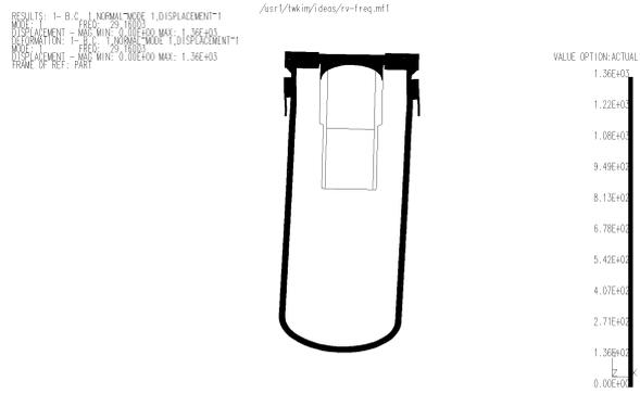
Fig. 3 1st mode shape of RV
