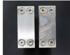
Fig 5. Heater surface from before and after the CHF test
