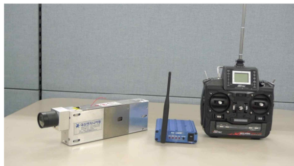
Fig. 2. A detailed view of the neutron guide visual inspection system.
