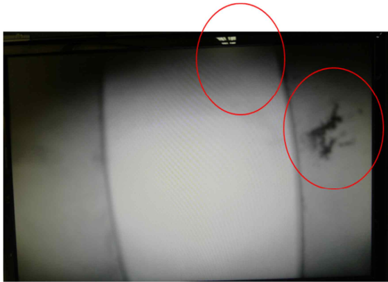
Fig. 4. A wide angle shot of NG Ni-coating exfoliations which are detected from NG visual inspection system.
