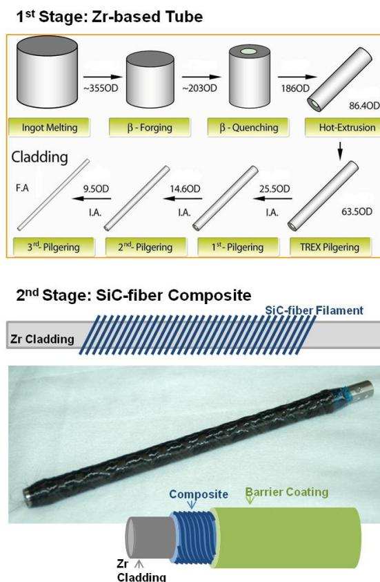
Fig. 1. Manufacturing process of the metal-ceramic hybrid fuel cladding tube. The first stage corresponds to the inner metal structure, and the second stage to the outer ceramic composite layer.
