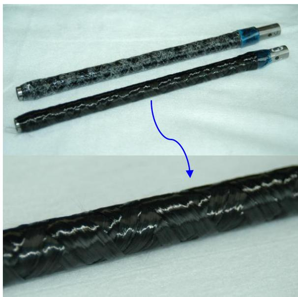
Fig. 2. Samples of metal-ceramic hybrid fuel cladding tubes after filament winding in dry (bottom) and wet (above) conditions.
