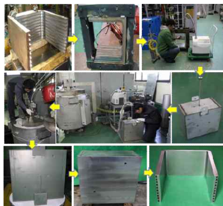
Fig. 1. Manufacturing process for a half-scale sub-module mock-up.
