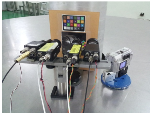
Fig. 1 Various CCD cameras take a front view of the gamma ray source (Co-60).
