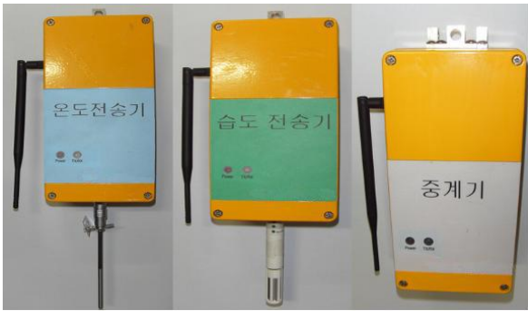
Figure 1. Wireless smart temperature and humidity sensors and repeaters
