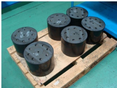
Figure 6. Natural rubber bearing for mechanical property test
