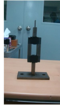
Figure 2. Test model for determining shear strain of rubber material
