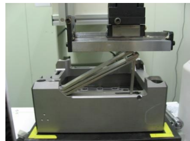
(b) Test Setup for One Holddown Spring Set Figure 1. Load vs. Deflection Test Setup
