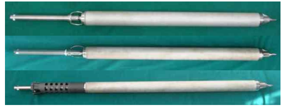
Fig. 2. Mockup devices (from top; 6-spring, 3-spring, and plug type) [3].
