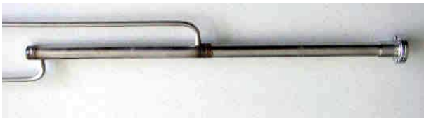
Fig. 1. Hydrogen concentration monitoring sensor.
