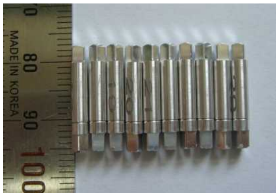
Fig. 3. The new type fluence monitors for 11M-20K and 11M-21K capsules
