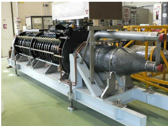
Fig. 1: Klystron for the PEFP 100MeV linac (TH2089K)
