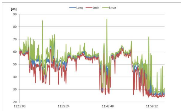
Fig. 5. Vibration effect by an excavator (Laeq: acceleration average level, Lmin: minimum level, Lmax: maximum level)
