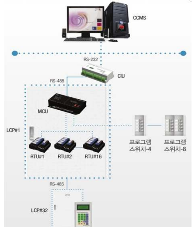
Fig 2. Monitoring System Configuration of Lighting Control System
