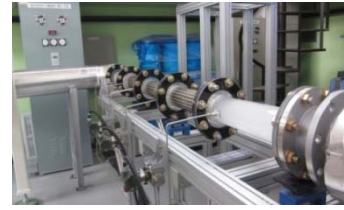
Figure 2-1 Test Column for Fuel Bundle
