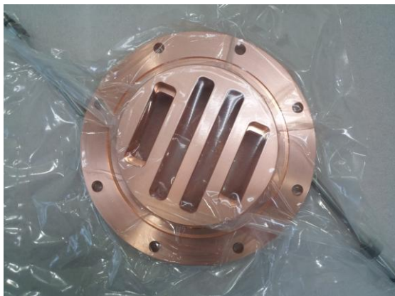
Fig. 6. Fabricated vacuum grill.
