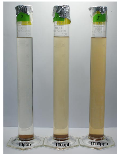
Fig. 2. Settling test results for different PAA concentration (10 & 1000 ppb). (a)just after dispersion, b)3h, c)24h, d)7 days suspension.)
