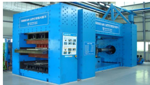
Fig. 1. The compression-shear test machine.
