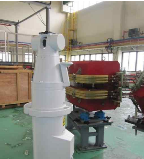
Figure 5. The fiducialization of a dipole magnet with a laser tracker.
