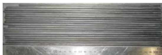
Fig. 1. Typical U-10%Zr-5RE fuel slugs, fabricated with the gravity casting furnace
