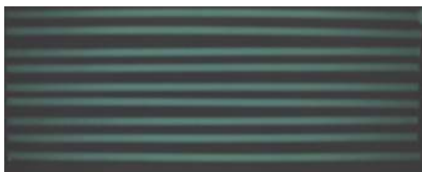
Fig. 2. Gamma radiography for internal defects detection of as-cast fuel slugs; U-10wt.%Zr-5RE.
