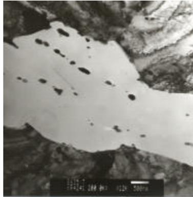
Fig. 4. Stringer of precipitates in Tube C
