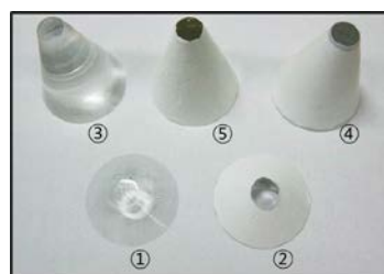
Fig. 5. Figure of the fabricated light guides
