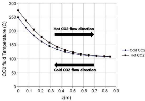
Figure 4. Results of temperature profile at the PCHE hot side and cold side conducted by Kim et al. [3].
