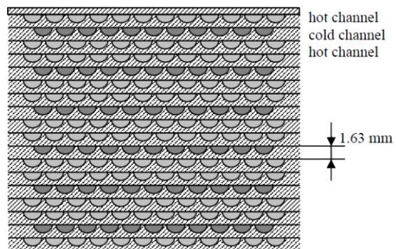
Figure 2. Cross-sectional shape of PCHE [1].
