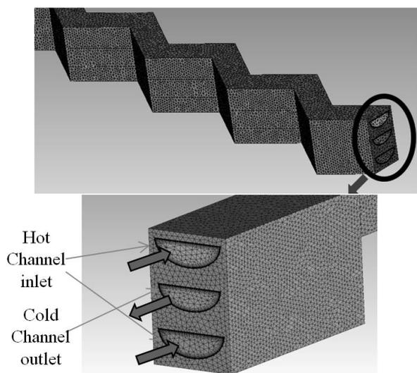
Figure 3. Grid shape of the PCHE analysis model
