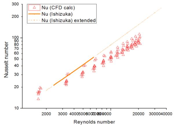
Figure 5. CFD results of Nusselt number in the hot side compared to the correlations.
