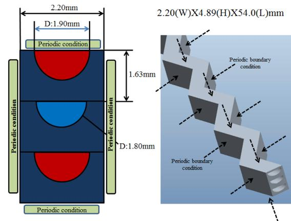
Figure 1. The geometry and boundary condition of PCHE analysis model.
