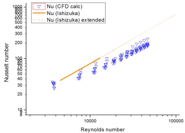
Figure 6. CFD results of Nusselt number in the cold side compared to the correlations.
