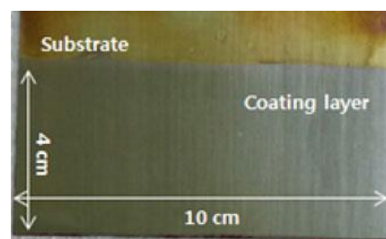
Fig. 4. The photograph of the electroplated Ni-63 on the Cu plate. The thickness of coated layer is to be 3 µm.
