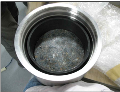
Fig. 4. Viton sleeve and concrete specimen in vessel
