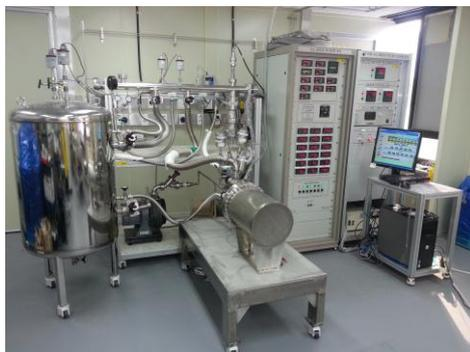
Fig. 1. DU bed hydriding/dehydriding system.
